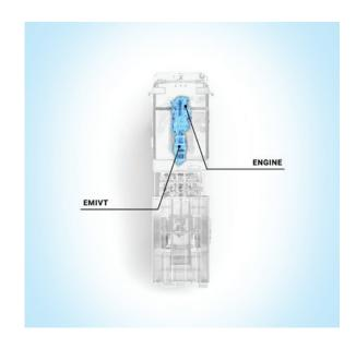
Because the EMIVT can also be coupled to the internal combustion engine, it will always provide continuous and uninterrupted power to the pumping system or drive system.
