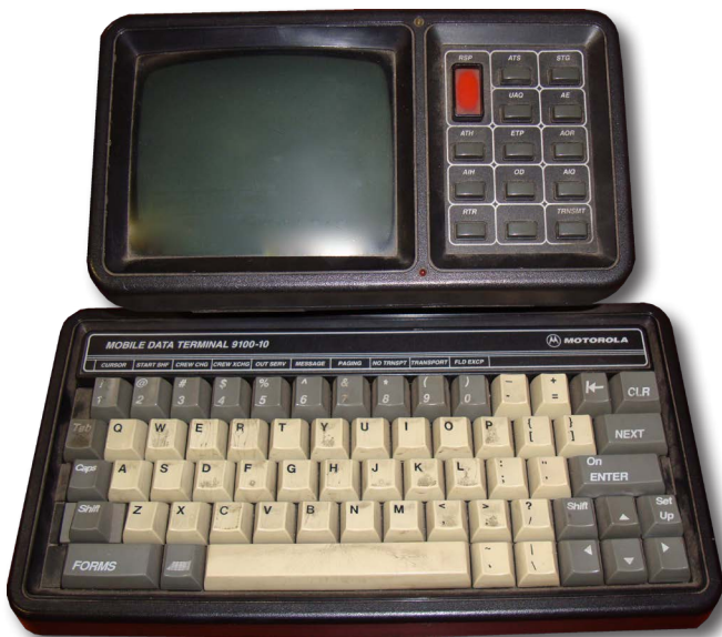
Figure 1-31 Mobile Data Terminals
