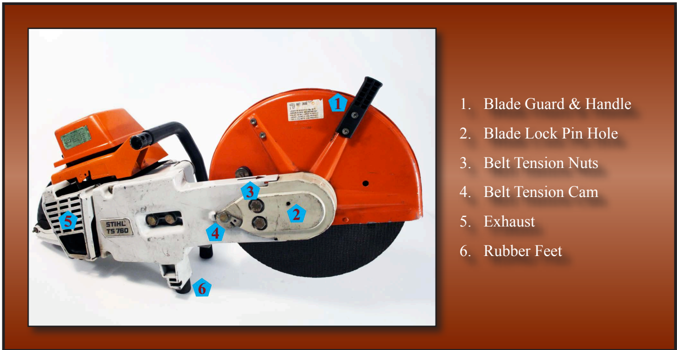
Figure 5-11 Right Side Rescue Saw Schematic
