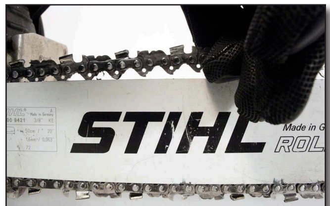
Figure 5-7 Proper Chain Tension
