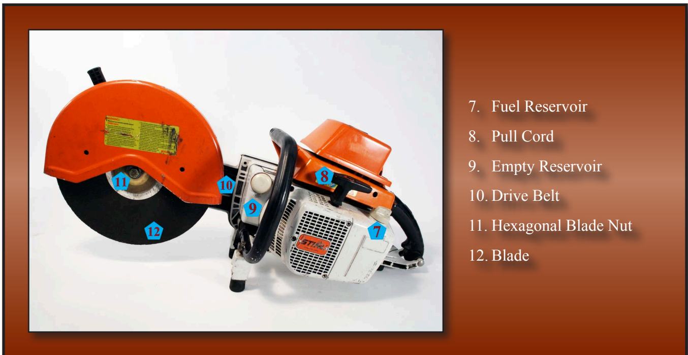
Figure 5-12 Left Side Rescue Saw Schematic
